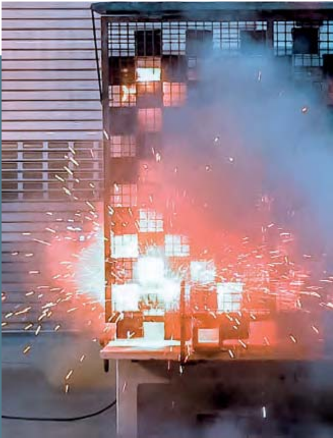
An arc short circuit resistance test I.
